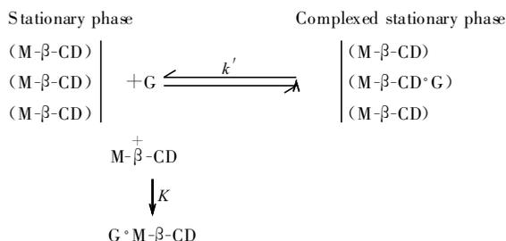
Fig 1. The equilibria system existing in methylated  $\beta$ -cyclodextrin dynamically coated chiral stationary phase proposed in reference<sup>[2]</sup>.
