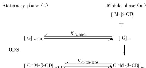
Fig 2. The equilibria system existing in the uncoated part on ODS surface with methylated  $\beta$ -cyclodextrin in the mobile phase.
